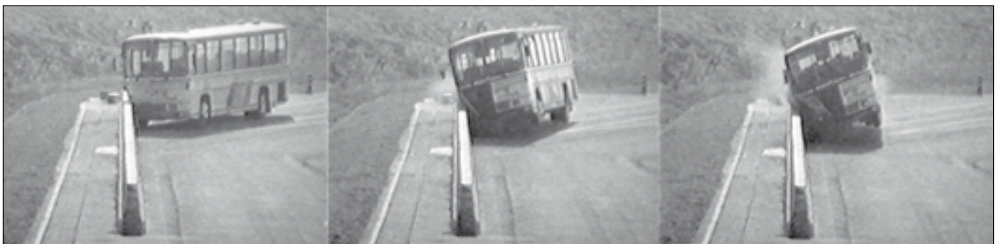
Tests on the new step barrier show how it controls a 13.5 tonne bus . . .
